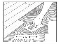
**NOTE**: Never work on top of the flooring when installing. If you must work on top of the newly laid flooring, use a kneeling board.
