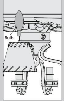
Install a light bulb in each socket.
