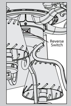
To switch the direction of air flow, move the reverse switch to the opposite position.
