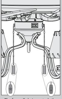
The fan pull chain controls the speed: from high to off.
