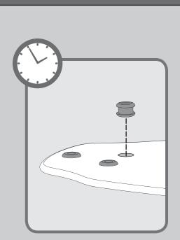
Time Saver Tip: Get a helper to insert grommets, found in the ■ hardware bag, into the blades while you're doing the next couple of steps.
