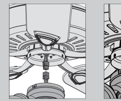
Connect the plugs from the upper and lower switch housings. Make sure to line up the colored markings on the connectors.
