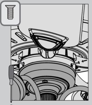
Insert three switch housing screws found in the  $\equiv$  hardware bag.
