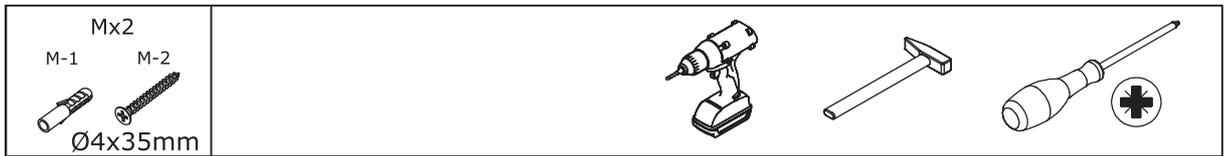
Install anti-tipping device(M) as shown.
