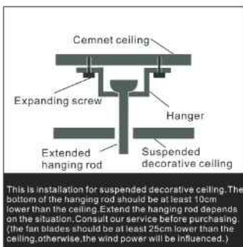
Diagram 3: Installation with suspended decorative ceiling
