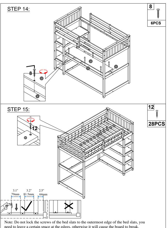
note: Do not lock the screws of the bed slats to the outermost edge of the bed slats, you need to leave a certain space at the edges, otherwise it will cause the board to break. Do not lock the bed slats on the edge of the wood, please hold firmly before screwing, hold it in place with one hand, then lock the screw.
