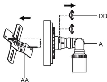
2. Attach cross bar (AA) to outlet box (not included) using outlet box screws (BB).
