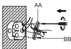
3. Strip 3/4 in. of insulation from fixture wire ends. Twist stripped ends together with pliers (not included), black to black (power), white to white (neutral). Snip ends. Wrap the ground wire from the outlet box around the green screw preassembled on the cross bar (AA), and then connect the ground wire from the outlet box to the ground wire from the fixture.
