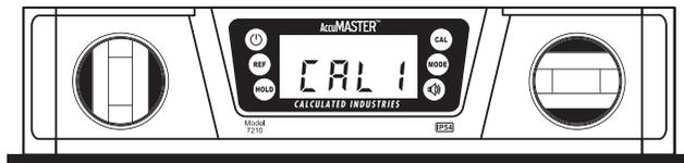
4. Rotate the level 180°, wait for 10 seconds until the display digits stop changing, then press the CAL button until "CAL2" displays. Once "CAL2" disappears, it indicates the user calibration is complete. The display will show the current angle.
