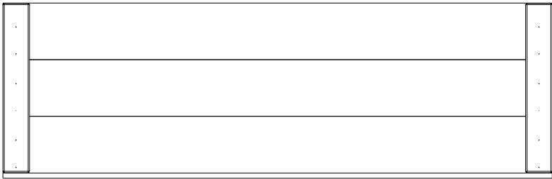
RP2 ROOF PANEL - W2A03947 (x2) 1 5/8"x15 5/8"x59 3/8" (42x396x1241)
