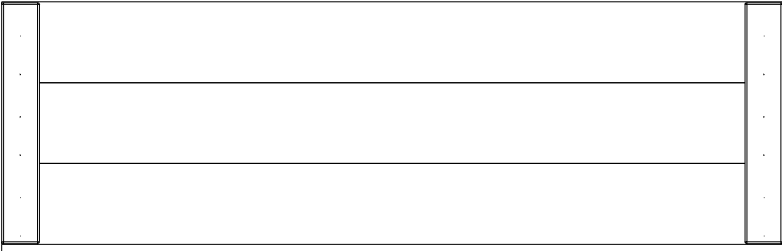
RP2 ROOF PANEL - W2A03947 (x3) 1 5/8"x15 5/8"x59 3/8" (42x396x1241)
