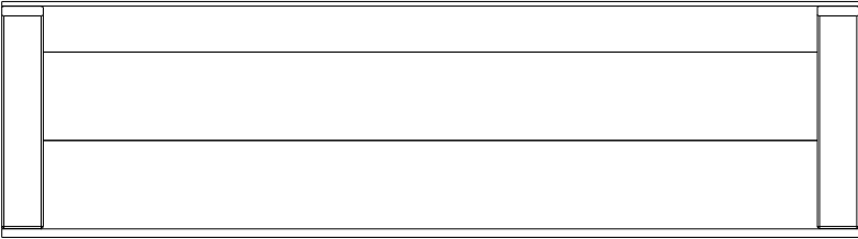
RP1 PEAK ROOF PANEL - W2A03948 (x2) 1 5/8"x13 3/8"x48 7/8" (42x341x1241)
