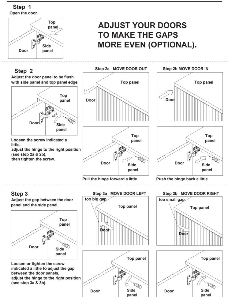
Turn the screw clockwise a little as shown to make the gap smaller
