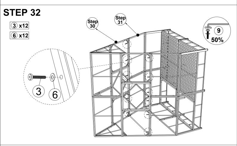
Connect The part from Step 31 & The part from Step 30, tighten Bolt (3) & Flat Washer (6) with Allen Key (9).
