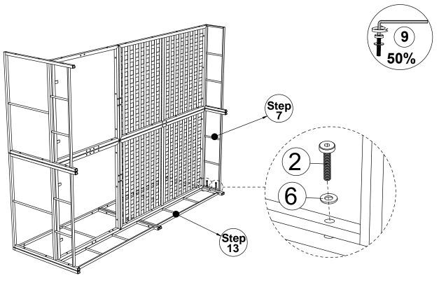
Connect the part from step 13 & the part from step 7, tighten Bolt (2) & Flat Washer (6) with Allen Key (9).
