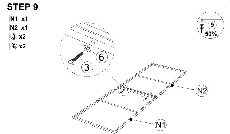
Connect Right Bottom Roof (N1) & (N2), tighten Bolt (3) & flat washer (6) with Allen Key (9).
