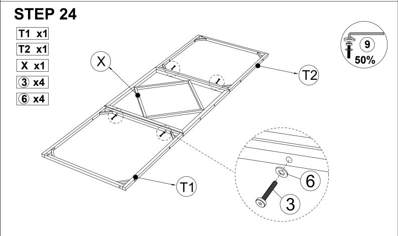
Connect Right Middle Roof 1 (T1) & 2 (T2) & Center Middle Roof (X), tighten Bolt (3) & Flat washer (6) with Allen Key (9).
