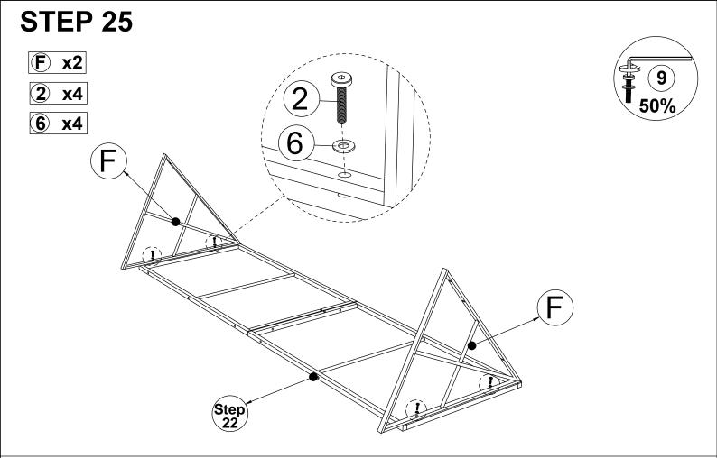
Connect a part from Step 22 & Triangle Roof (F), tighten Bolt (2) & Flat Washer (6) with Allen Key (9).
