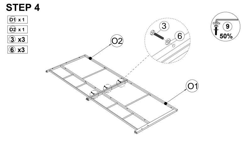
Connect Left Side Leg (O1) & (O2) With tighten Bolt (3) & flat washer (6) with Allen Key (9).
