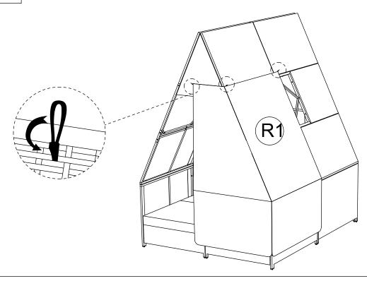
Connect Curtain 1 (R1) outside around the roof, sticked by plastic detail on Curtain
