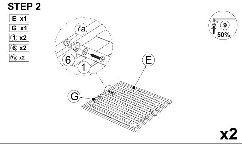
Connect Back Rest Frame (E) & Lifting Set (G) with tighten Bolt (1) & flat washer (6) ,Plastic Washer (7a) & Allen Key (9).
