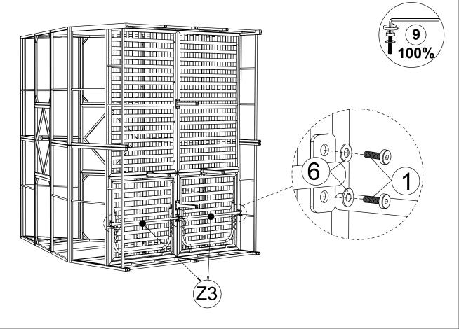
Connect The part from Step 34 & Support Bar (Z3), tighten Bolt (1) & Flat Washer (6) with Allen Key (9). Turn the final part upright.
