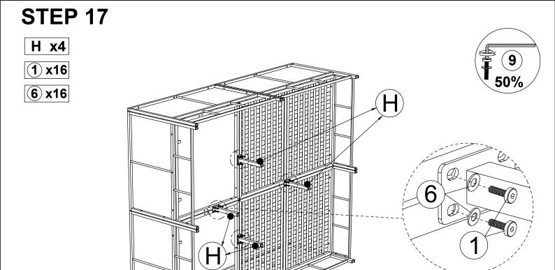
Connect the part from step 16 & Support Leg (H), tighten Bolt (1) & Flat Washer (6) with Allen Key (9).
