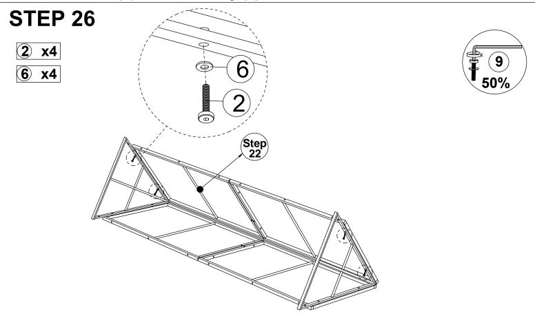
Connect the part from Step 25 & the last one from Step 22, tighten Bolt (2) & Flat Washer (6) with Allen Key (9).
