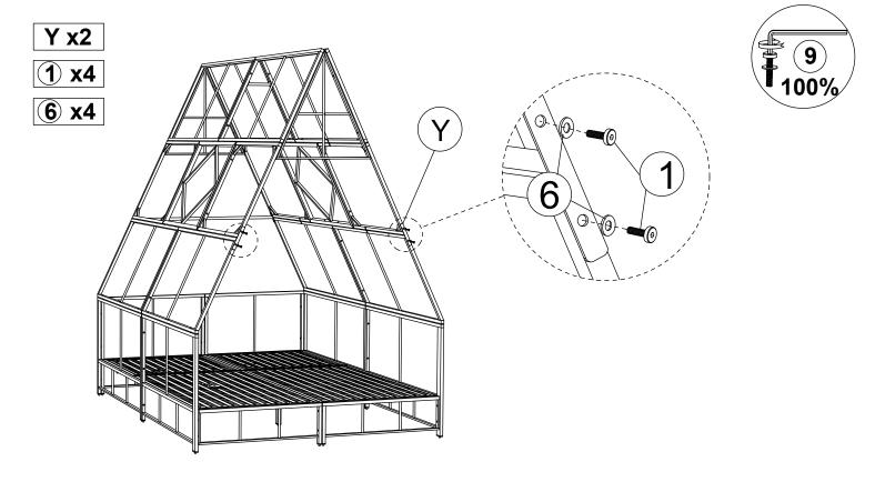
Connect The part from Step 36 & Connecting Flat (Y), tighten Bolt (1) & Flat Washer (6) with Allen Key (9).
