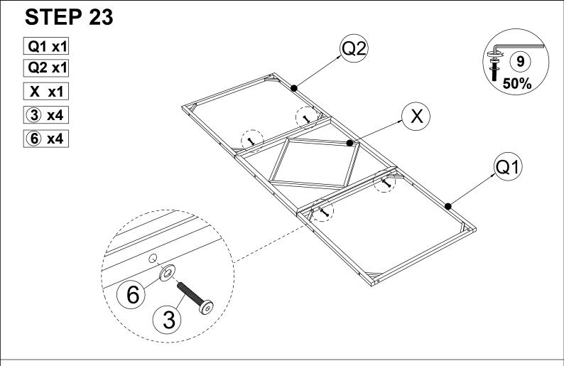
Connect Left Middle Roof 1 (Q1) & 2 (Q2) & Center Middle Roof (X) With tighten Bolt (3) & Flat washer (6) with Allen Key (9).
