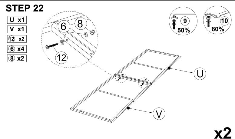
Connect Top Roof 1 (U) & Top Roof 2 (V), tighten Bolt (12) & Flat Washer (6), Nut (8) with Allen Key (9).
