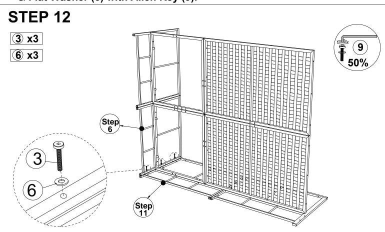
Connect the part from step 11 & the part from step 6, tighten Bolt (3) & Flat Washer (6) with Allen Key (9).
