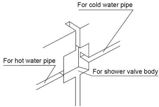
① Use special tools to chisel holes on wall for installing, shower valve body and water pipe.
