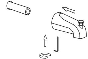
⑧ Wrap some plumber's tape on the internal gut, and screw the bathtub spout. Switch to the top spray by lifting the switch on the spout when use.
