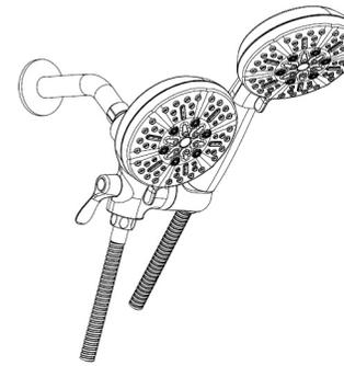
⑦ Place hand-held shower head in rotatable holder. Point all shower heads away from you and turn on the water full force. Check for leaks. Re-tighten all connectors if necessary.
