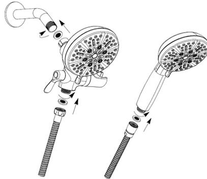
⑥ Attach 3 in 1 fixed mount shower head by threading clockwise onto shower arm with rotatable holder to the right and 3-way diverter control handle to the left. Use a wrench to tighten shower head nut to a properly snug fit. Then connect the shower hose to the shower head and hand shower as the pictures shows.
