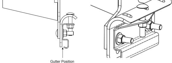
Position the cross member to desired position and tighten the two nuts to 17 ft-lb. Vertically constrain the inverted J-bracket and the gutter clamp using one 1-3/4" carriage bolt, washer, and a nut.
