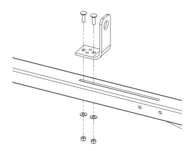
STEP 4A. MOUNT CROSS MEMBERS TO VEHICLE - (Ford Transit, Nissan NV, and MB Sprinter) Slide two stud plates per mounting channel if not already done. Lift the assembled ladder rack and place it on the stud plates on all four corners. Use (2) washers, (2) nylon lock nuts, and a bolt plate to fasten each mounting foot.
