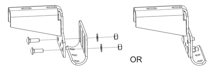
STEP 1B. LOOSELY ASSEMBLE GUTTER MOUNT CLAMP AND J-BRACKET TO UNIVERSAL MOUNTING BASE (GMC Savana / Chevy Express, and Ford E-Series)
