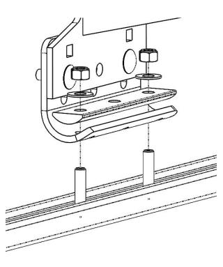
STEP 4B. MOUNT CROSS MEMBERS TO VEHICLE - (GMC Savana / Chevy Express, and Ford E-Series) Make sure that the gutter is clamped between the gutter clamp and the inverted J-bracket.
