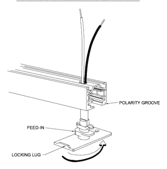
INSERT WIRE AND LIVE FEED-IN THRU HOLE IN TRACK WITH POLARITY GROOVE ON THE OPPOSITE SIDE OF THE LOCKING LUG. TURN LIVE FEED IN A CLOCKWISE DIRECIION FOR 90° TO LOCK INTO POSITION. (SUGGEST YOU USE A LARGE PAIR OF PLIERS WITH CAUTION SO THAT YOU DO NOT SCRATCH THE TRACK OR DAMAGE THE EDGE OF LIVE FEED-IN UNIT).
