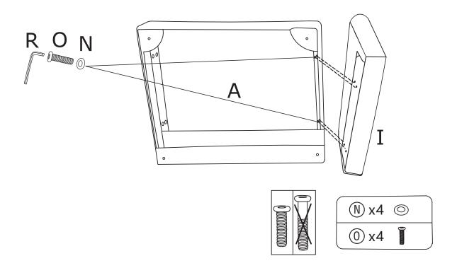
STEP 3: Assemble Seat frame (A) and Seat frame (A)with Butterfly nuts (Q) Washers (N) and Bolts (P).
