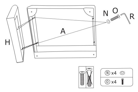
STEP 2: Assemble the Right armrest (I) to the Seat frame (A) with Washers (N) and Bolts (O).
