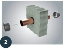
Install pipes or cables. Install backing material as required into annular space as shown to both sides of wall assembly.
