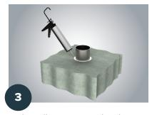
Apply caulking as required to close remaining gap to both sides of floor assembly; providing a smoke and gas resistant seal. Spread caulking smoothly and evenly all around.
