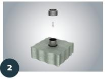
Install pipes or cables. Install backing material as required into annular space as shown to both sides of floor assembly.
