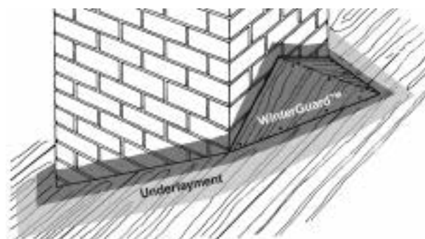
Figure 6-8: Chimney through the roof deck.
