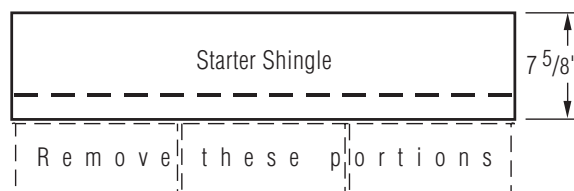
Figure 12-5: Make starter shingles that are 7 5/8" in height.
