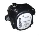
• Suntec/Webster Fuel Pump: Single stage fuel pump will push the waste oil 25 ft. vertical, and 100 ft. horizontal. (Always run fuel lines up to the burner, never down, or you could create an air pocket in the system – Hard to Bleed)
