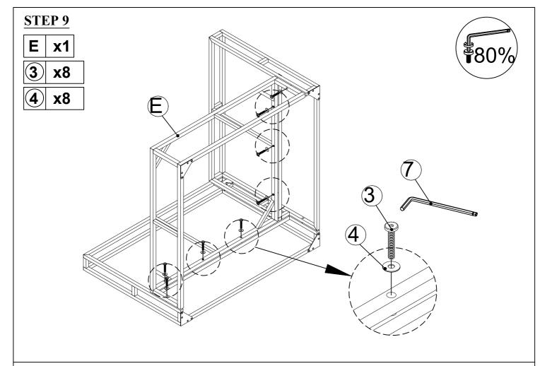
Connect Connect the part from step 8 with Seat Conner (E), Tighten Bolt (3) & Flat Washer (4) with Allen Key (7).
