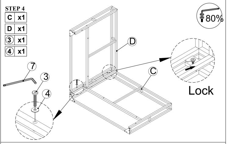
Connect Back Left Conner (C) & Hand Left Conner (D), Tighten Bolt (3) & Flat Washer (4) with Allen Key (7).
