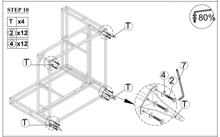
Connect Connect the part from step 9 with Leg (T), Tighten Bolt (2) & Flat Washer (4) with Allen Key (7).
