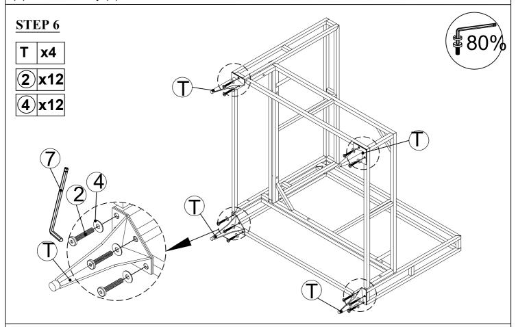
Connect Connect the part from step 5 with Leg (T), Tighten Bolt (2) & Flat Washer (4) with Allen Key (7).
