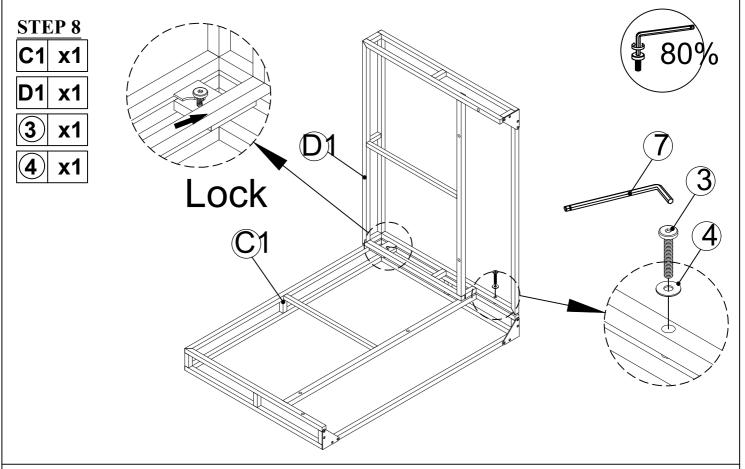
Connect Back Right Conner (C1) & Hand Right Conner (D1), Tighten Bolt (3) & Flat Washer (4) with Allen Key (7).
