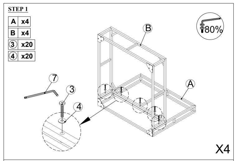
Connect Seat Chair (B) & Back Chair (A), Tighten Bolt (3) & Flat Washer (4) with Allen Key (7).
