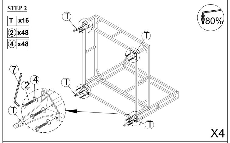
Connect the part from step 1 with Leg (T), Tighten Bolt (2) & Flat Washer (4) with Allen Key (7).
