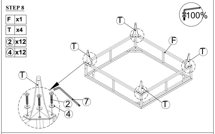
Connect Top Table (F) with Leg (T), Tighten Bolt (2) & Flat Washer (4) with Allen Key (7).
