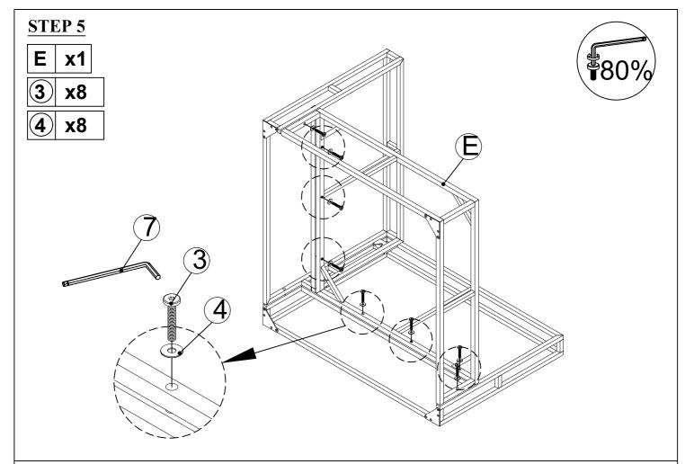
Connect Connect the part from step 4 with Seat Conner (E), Tighten Bolt (3) & Flat Washer (4) with Allen Key (7).
