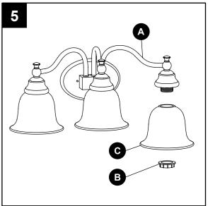
Install light bulbs (not included). Use 60-watt max. standard-base incandescent bulbs or halogen/ CFL/LED equivalents.
