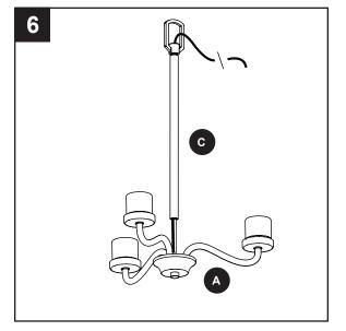
If desired, use pliers (not included) to open chain links to shorten the chain (D). Then open the connecting links (F) by twisting the nut and connect to each end of the chain (D). Attach the connecting link (F) at the bottom of the chain (D) to the decorative tube (C).
