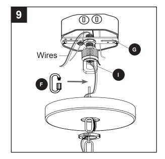
10. Twist nut to close connecting links (F) at each end of chain (D).
