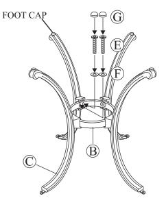
Place the table top upside down on a flat, nonabrasive surface. Attach table leg to table top using a 1/4"x18 mm bolt and washer as shown in the diagram. Guide bolt through hole in table leg, into pre-drilled hole in the table top. Hand tighten three to four turns only. **Do not tighten completely**. Some adjustments may be necessary to ensure proper alignment of the table legs. Repeat for the other three legs.
