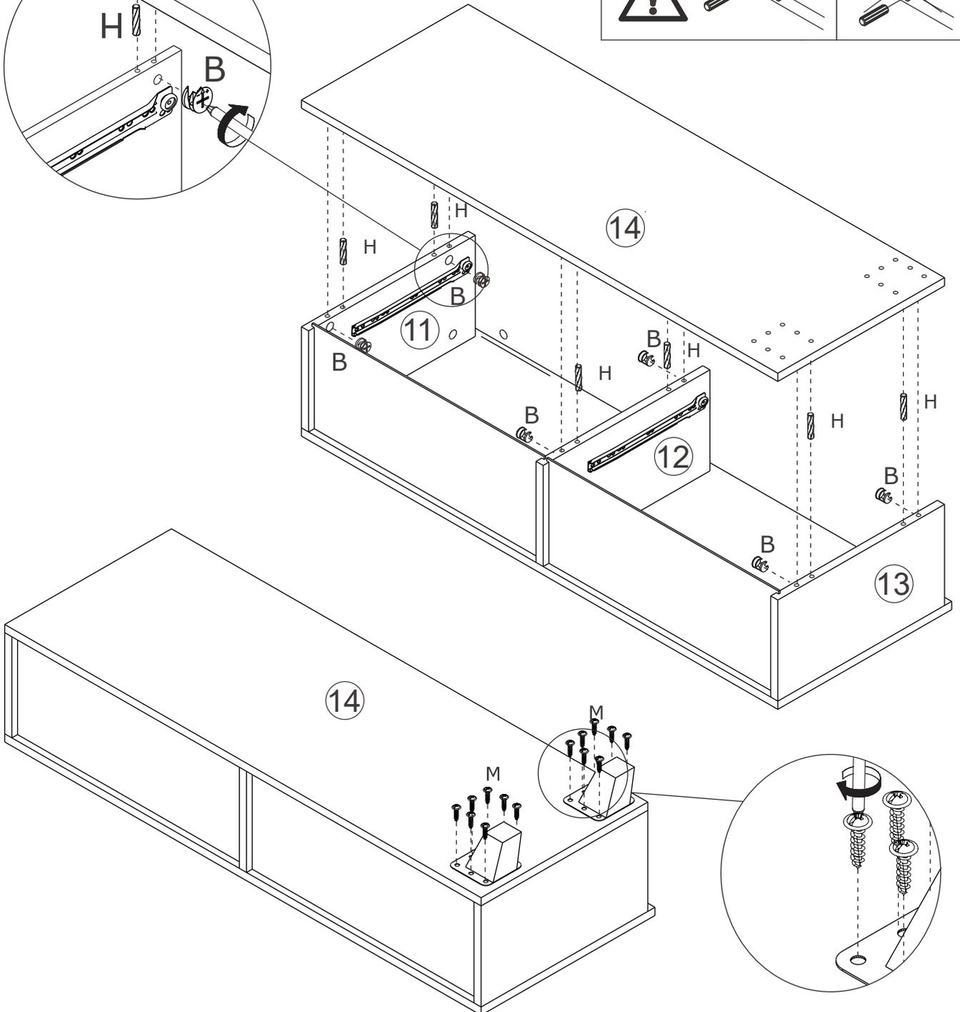
As shown in the figure, insert No. H wooden tenon at the corresponding reserved holes on No. 11, No. 12 and No. 13 plates, cover No. 14 plate, and put in No. B eccentric wheel to rotate 90-180 degrees clockwise; Finally, connect the foot of the TV cabinet to the cabinet body with the M screw.
