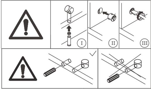
As shown in the figure, insert No. H wooden tenon at the corresponding reserved holes in No. 11, No. 12 and No. 13 plates, then cover No. 15 plate and put in No. B eccentric wheel to rotate 90-180 degrees clockwise; Finally, connect the foot of the TV cabinet to the cabinet body with the M screw.
