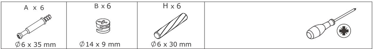
As shown in the picture, fix No. A screw and No. H dowels to the reserved holes on No. 9 board and insert No. 11, No. 12 and No. 13 boards (the grooves are on the same side).
