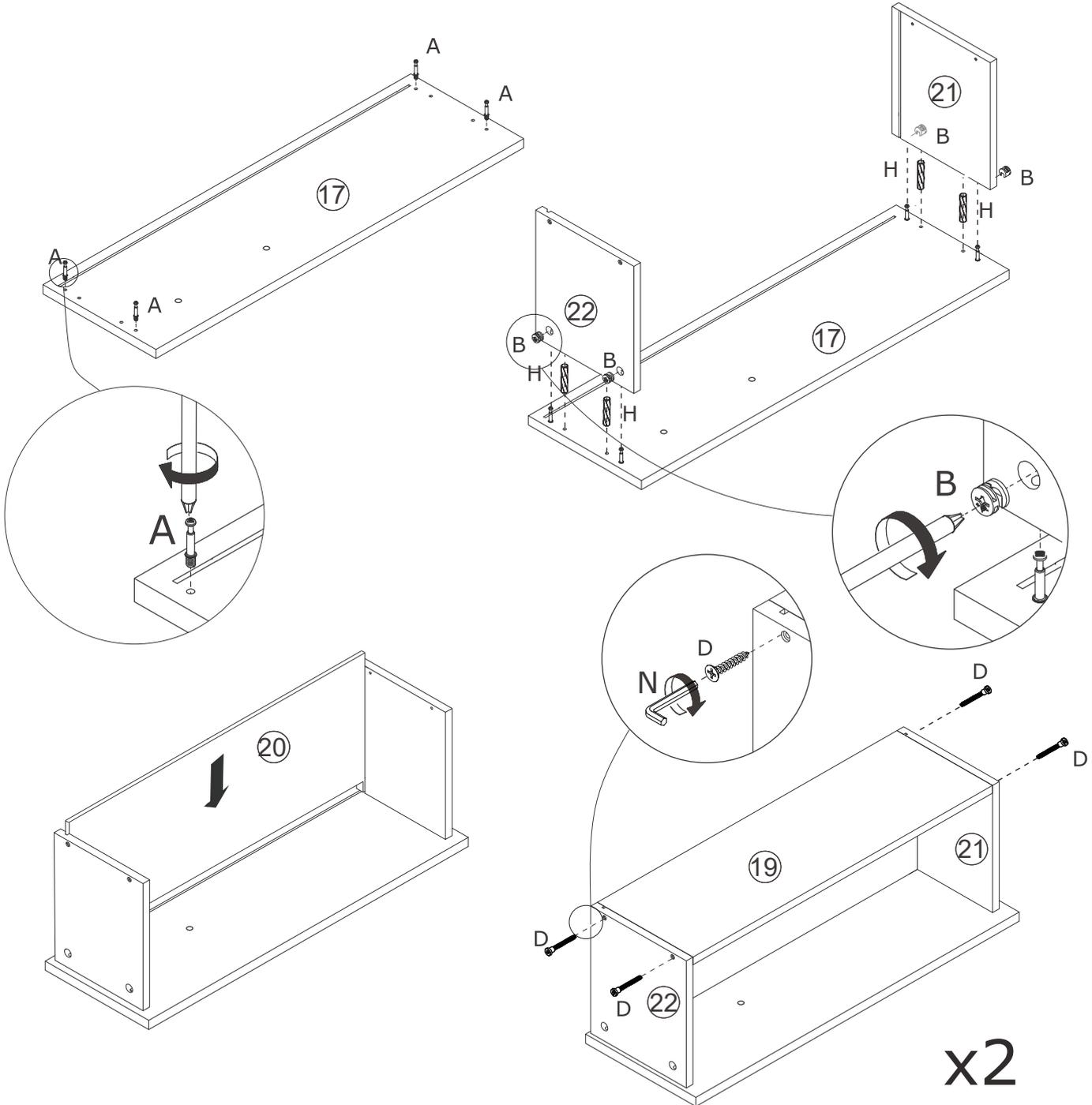
As shown in the picture, fix No. A screw and No. H wooden tenon No. 17, insert No. 21 and No. 22 plates, put in No. B eccentric wheel and rotate clockwise 90-180 degrees; Then insert No. 20 sheet and connect No. 19 plate to No. 21 and No. 22 plate using No. D screw and No. N wrench.
