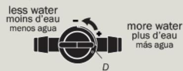
c) Repeat 7b until bowl water level reaches pencil mark at the same time tank finishes filling.
