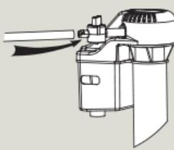
Tip: Run tube under warm water for easier install.
