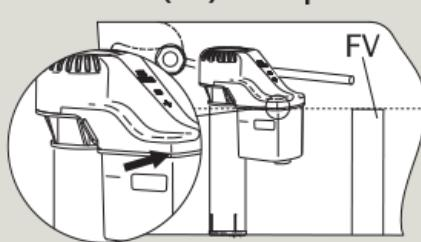
Tip: If tower style flush valve (TS), match fill valve water line to water line marked in tank (stain line).
