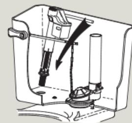
**3 a) Press down until corner of silver cover and top of flush valve (FV) line up.**
