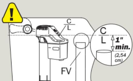
b) Attach tube to flush valve (FV) with metal clip so water flows into flush valve. Trim tube if kink occurs.
