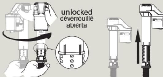
**c) Place valve in tank.**
