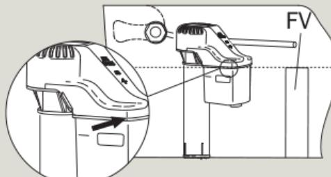
**c) Install mounting nut. Hand tighten only, beveled side up.**
