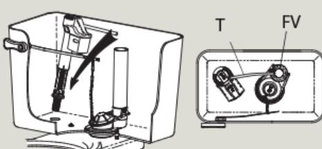
**b) Verify corner of silver cover and top of flush valve (FV) line up.**
