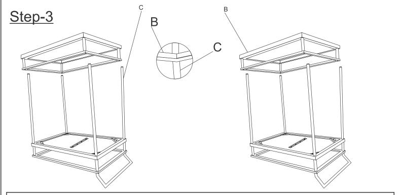
Put the panel (B) in such a way that it will coincide with item (C) at all four corners perfectly.
