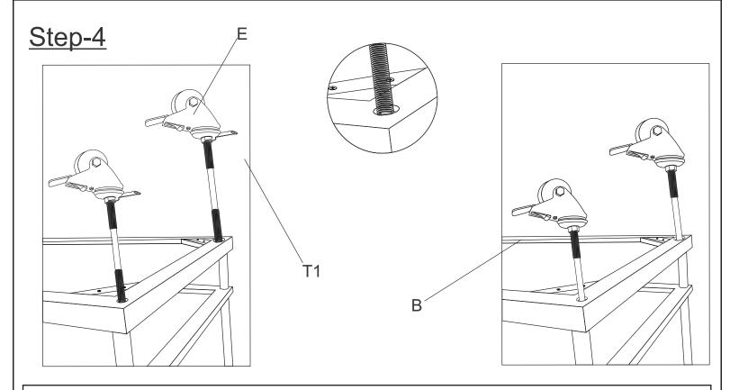
Insert the rod of item (E) into the panel (B) and get it screwed the help of item (T1) all four corners.
