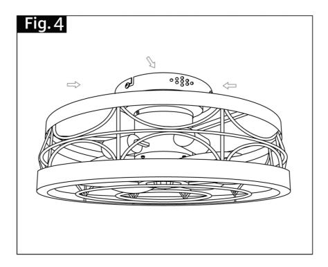
Place the two key holes from the ceiling fan over the two screws previously loosened from the hanging bracket. Turn the ceiling fan until it locks in place at the end of the key holes. Secure by tightening the two screws previously loosened and the one screw previously removed.
