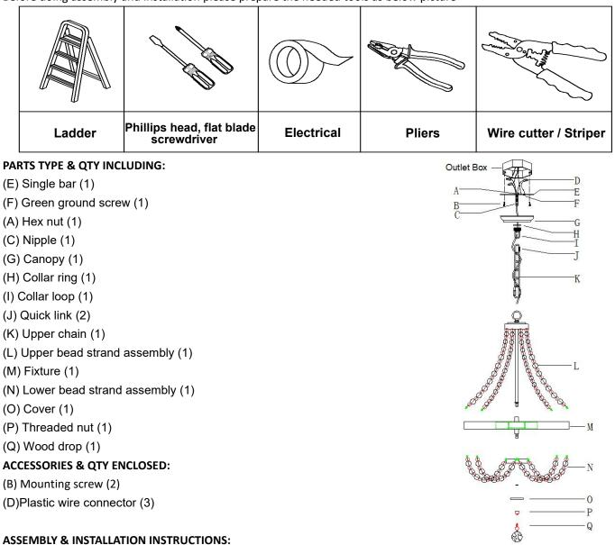
1. Carefully remove the fixture from the carton and check that all parts and accessories are included as shown in the above illustration
