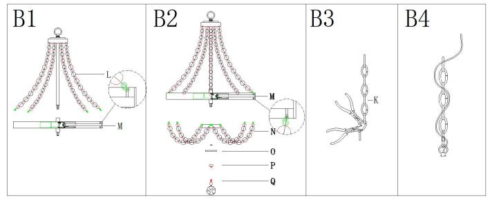
Step B1: Thread the fixture (M)onto the threaded nipple on the fixture body (M) Carefully hang the bead strands onto the fixture body (M)
