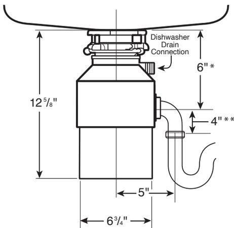
\* Distance from bottom of sink to center line of disposer outlet. Add 1/2" when stainless steel sinks are used.
