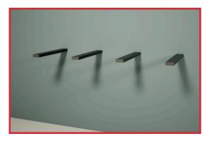
3. Install drywall to your wall studs. Ensure your drywall is cut to fit around your brackets. Cut out a 2.5" wide by 1" deep notch from your drywall with each bracket
