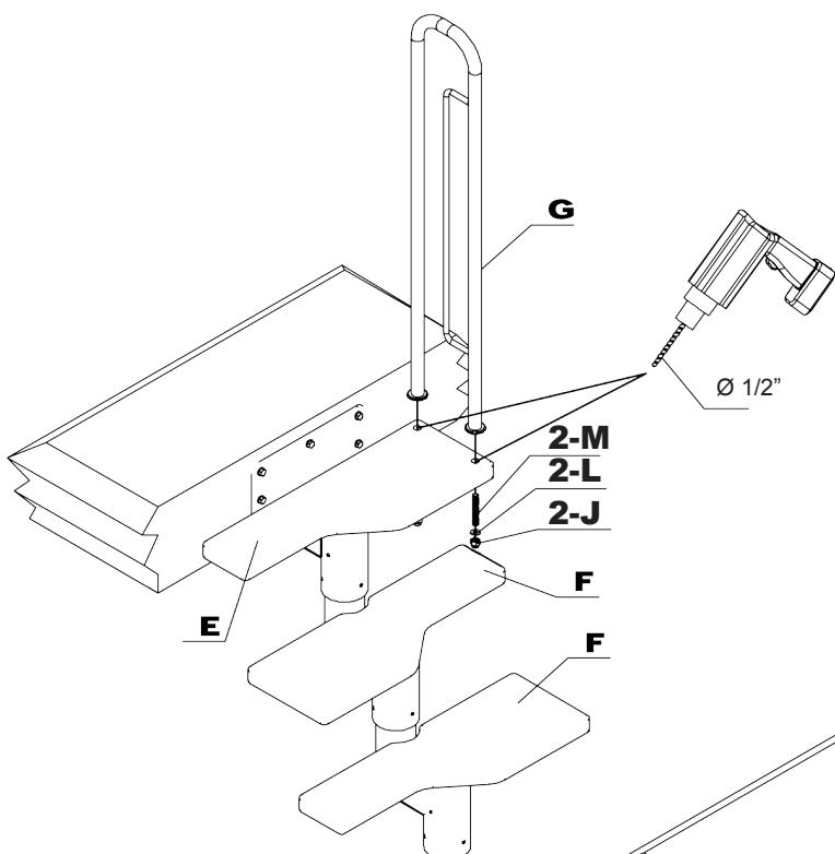
Measure distance of top tread and cut banister to appropriate length - **CC**.
