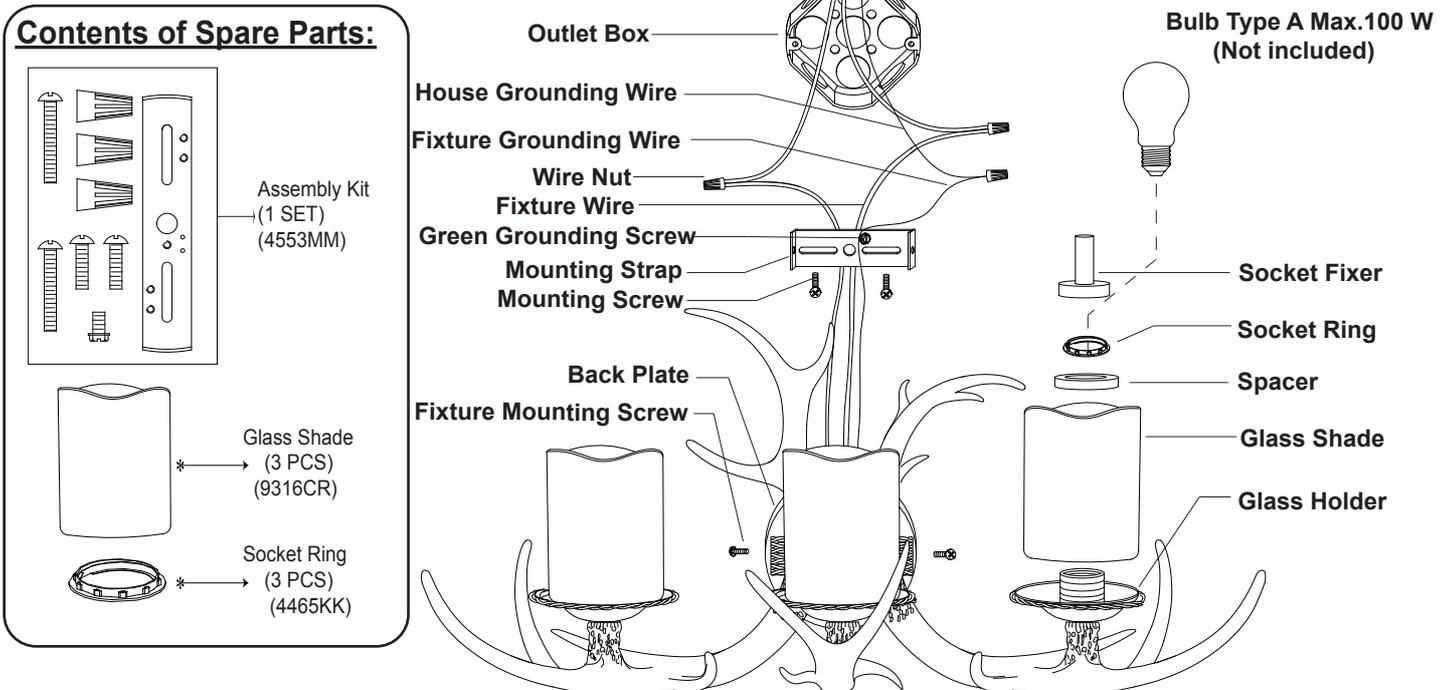
1. Attach the mounting strap to the outlet box by using two mounting screws.
