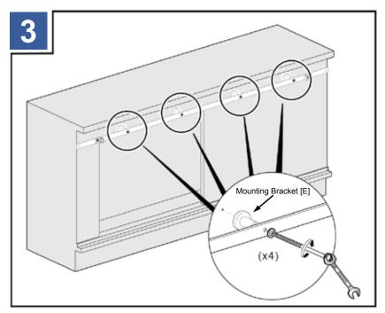
Install the rail, and mounting brackets [E].
