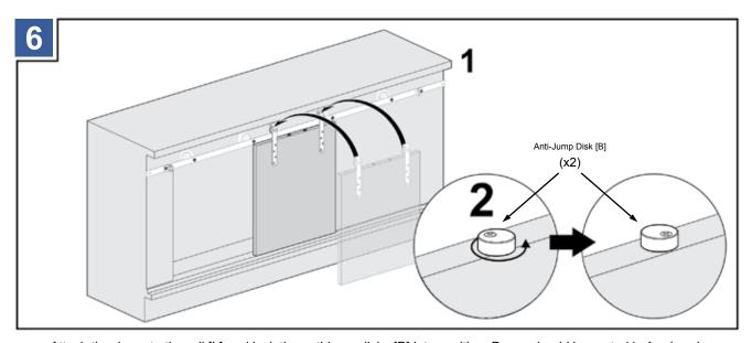
Attach the doors to the rail [L] and lock the anti-jump disks [B] into position. Doors should be routed beforehand if using the routed door guides [G].
