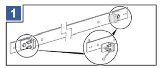
Before beginning installation, attach the door stops [C] to the rail [L].
