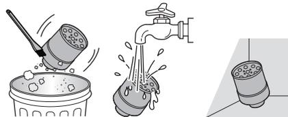
**6** Use the combination tool **5** to clean out dust or foreign objects inside the dust bin.
