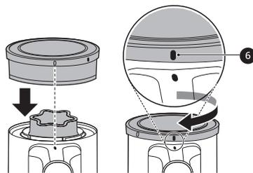
**8** Align the lock position fo **6** the exhaust filter cover with the letter "H" **7** of the **PUSH** button on the exhaust filter.
