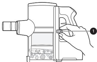
**3** Press the dust bin cover release button **2** to open the dust bin cover. Shake the dust bin to empty it.
