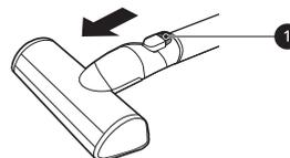
**2** Turn the nozzle upside down and rotate the cover lock slot **2** counterclockwise.
