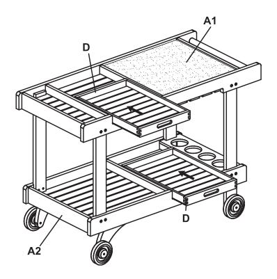
Attach the trays (D) to the section Top frame (A1) and bottom frame (A2). THE TROLLEY CART IS NOW READY FOR USE.
