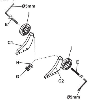
Attach wheel (I) on to right & left bottom leg (C1&C2). Insert 3" Bolts (E), Washer(H), and nut (G) hold on the bolts using Ø5mm Allen wrench, and tighten nut using wrench.
