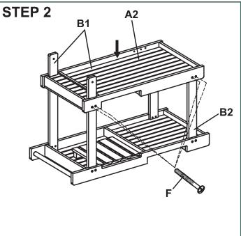
Attach long legs (B1) and short legs (B2) on to top frame (A1). Insert 1 1/2" Bolts (F) using screwdriver. As picture shown.
