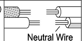
Twist wires together with plastic wire connector until tightly joined, and wrap each connector with approved electrical tape. Be sure that no wire strands are exposed and then carefully tuck all wires into the outlet box.
