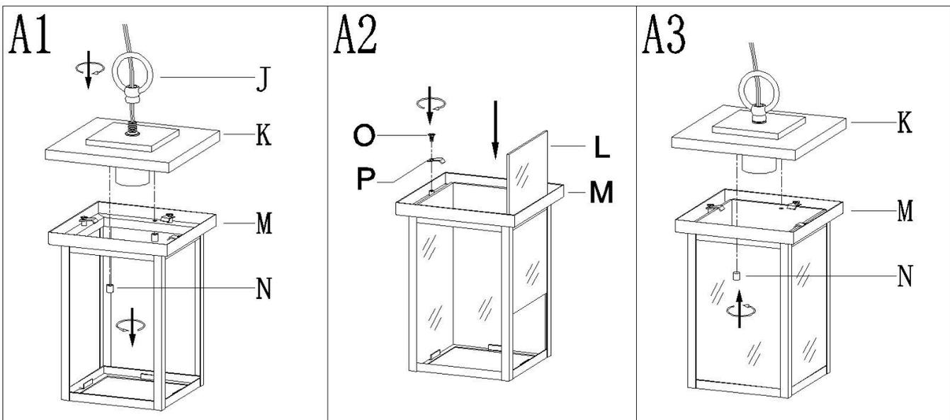
Step A1: Fix the loop (J) on the top of the cover (K).
