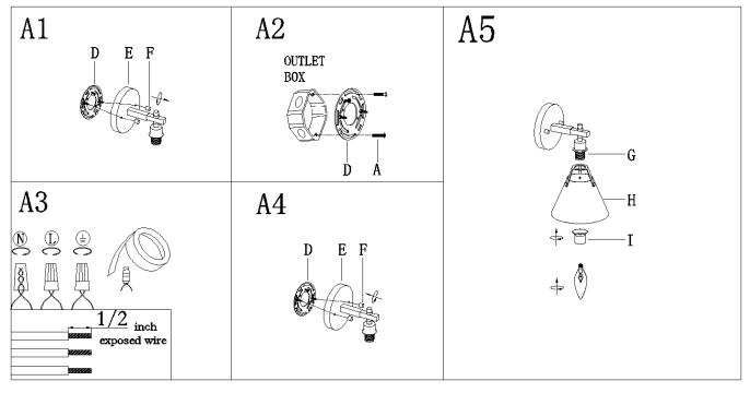
Step A1: Unscrew the ball knobs(F) from the back plate(E) then gently remove the mounting plate (D). Step A2: Secure mounting plate (D) to outlet box with mounting screws (A).
