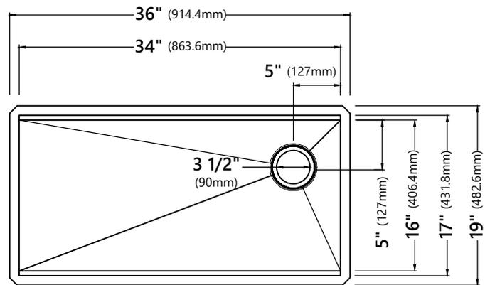
**NOTE:** It is not recommended to install this sink with a negative reveal. Doing so will prohibit the use of any workstation accessories as they will not fit.
