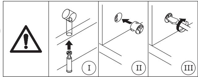
Insert wooden dowel(F) into the top of No.2 and No.3 plate as shown.
