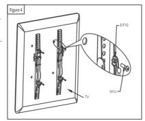
5. Adjusting your tilt: To adjust the tilt position on your display you will need to loosen the knob on the side of each one of the arm brackets. Due to the narrow space between your display and the wall it is recommended to first adjust the tilt while you have the display face down on a soft surface such as a bed. Once the knobs are loosened adjust them to the desired position. After you have set the tilt position tighten the knobs on the arm brackets then proceed to Step 6.
