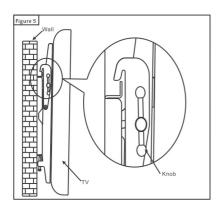
6. Attaching your display to the wall plate: This step may require two people, next you will attach your display to the mount. Take your display and lift it until the hooks set securely into the top lip of the mount (See Figure 5).
