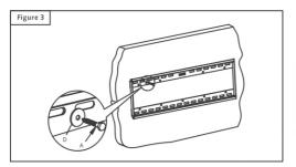
3. Attaching the mount to your wall: Once the four holes are pre-drilled fix the wall plate to the wall with all four lag bolts into the wall (See Figure 3). The included plastic anchors DO NOT need to be used for wood stud installation.
