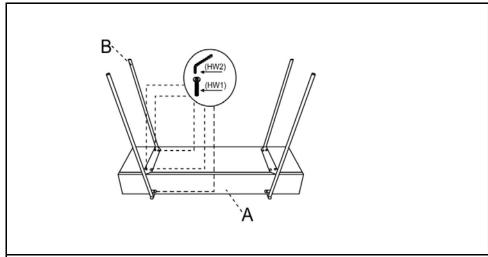
STEP1:Attach the legs(B) to the top(A), using Socket Screw(HW1), Tighten with allen key(HW2)
