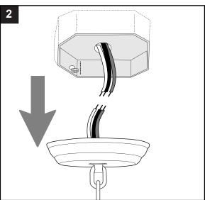
Attach mounting strap (C) to outlet box (not included) using the existing washers and outlet box screws or the machine screws (BB).
