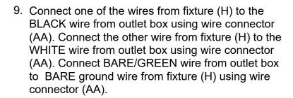
**NOTE:** If outlet box does not have a BARE/GREEN wire, the BARE ground wire from fixture (H) should be attached to the GREEN SCREW (labeled GND) on mounting strap (C).
