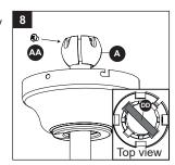
Slide the accessory downrod (sold separately) into the yoke of the ceiling fan. Install the accessory downrod according to the instruction manual included with the ceiling fan.
