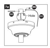
With the mounting bracket (B) resting inside the canopy (C), partially install two mounting bracket screws (EE) into the two holes surrounded by the J-slots in the canopy (C). Then, remove the mounting bracket (B) from the canopy (C).
