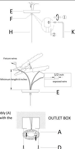
Twist plastic wire connector(C) until wires are tightly joined together, wrap each connector with approved electrical tape for more secure connection and carefully stuff all wires into the outlet box
