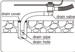
Insert the drain-pipe to the drain-hole on the floor, and then cover it with water retaining cover to prevent waste water spilling.
