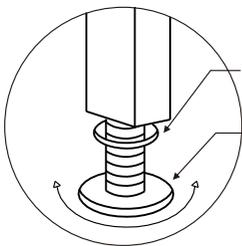
2.Adjust screw nut to the level position
