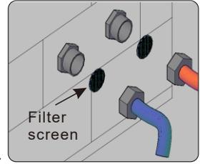
Before connect bathtub water inlet pipe, first open water pipe for a period of time, then put filter screen to ensure that the debris will not enter the bathtub pipe. So that we can effectively extend the life of the fitting.
