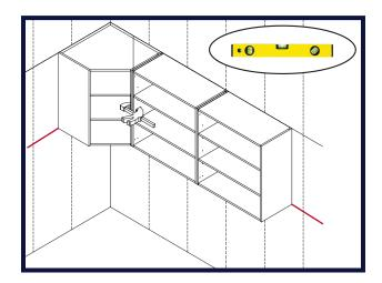
7. Set the next cabinet tight to the first cabinet and use clamps to hold in place while you level it and make sure that the front edges are flush. Attach the two cabinets together using 1 1/8" particle board screws. Attach the cabinet to the wall with 2 1/2" screws into the studs. Continue with the same process for all upper cabinets.
