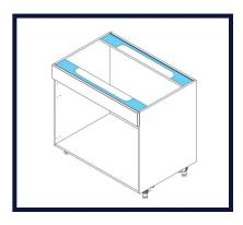
When installing a sink or cooktop, trimming the top support rails may be necessary. Using the template supplied by the sink or cooktop manufacturer, cut the top rails as required using a jigsaw.
