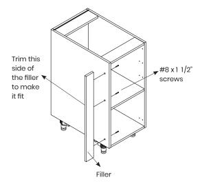
**Dishwasher Gables -** Measure 24 1/8" over from the cabinet at the front and the back and draw a line on the floor. Draw a plumb line on the wall from the floor to the base cabinet line. These lines mark the position of the inside of the dishwasher gable. Install a ledger board 24 1/8" long below the base cabinet guideline. The panel is then installed by attaching it to the ledger strip, floor and countertop with metal L-brackets.
