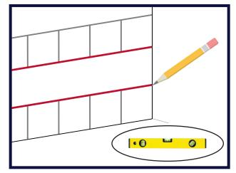
4. Draw a level line at 34 1/2" from the highest point of your floor and another level line at 54" from the same point. Install the top of the base cabinets level with the 34 1/2" line by using the adjustable legs to level the cabinets. Install the bottom of the wall cabinets level with the 54" inch line.
