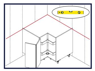
8. Always start with the corner base cabinet making sure it is level. Install 2 1/2" screws through the top fastening strip into the studs that were previously marked.
