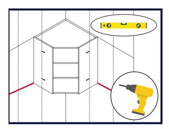
5. Starting with the corner wall cabinet, install (x4) 2 1/2" cabinet screws through the fastening strips on the cabinet into the wall studs. Be sure to check for level before fastening the cabinet into place.
