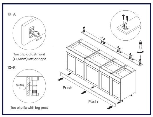
10. To install the toe kick clips, push the clip onto the top of the toe-kick as shown in step 10-A and step 10-B. To install the toe-kick, insert the top first and then push at the bottom to make a tight fit.
