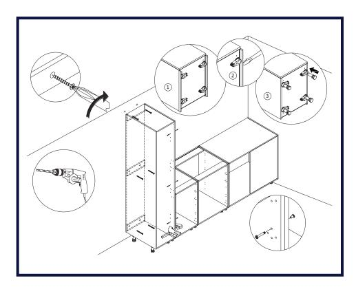
13. When installing tall cabinets, make sure they are level and plumb. Attach to studs, using 2 1/2" screws into all studs at the top, middle and bottom, screwing through the hanging rails. If the tall cabinet is against other cabinets, use your clamps to hold it place and screw the cabinets together using 11/8"screws.
