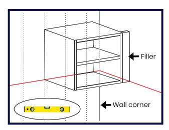
6. If you do not have a corner, start with the end closest to a wall, making sure to leave room for the required filler, as per your plan.
