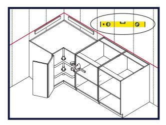
12. For designs with a corner cabinet, set the next cabinet tight to the first cabinet and use clamps to hold it place while you level it, and make sure that the front edges are flush. Attach the two cabinets together using 1 1/8" particle board crews. Attach the cabinet to the wall with 2 1/2" screws into the studs. Continue with the same process for all base cabinets.
