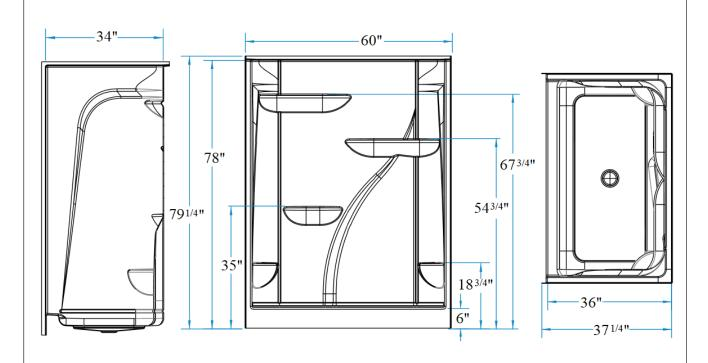
FEATURES lbs Dimensional Tolerance ± 3/8". Dimensions needed for site preparation should be measured from the unit.
