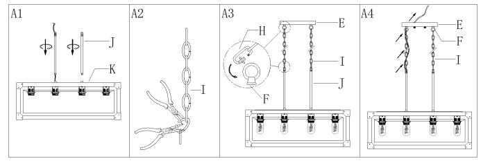
Step A1: Slip the tube (>) along wires then thread onto the nipple of top fixture body (?) till snug ,thread another tube(>) onto the nipple of top fixture body (?) till snug.
