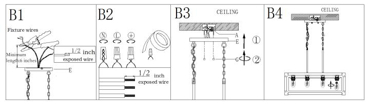
Step B1: If needed, cut off the wires length of fixture.At this point, the remaining wire length measured from the top center of canopy (E) is at least 6".
