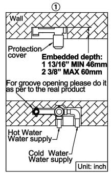
1. Make a groove in the wall as shown, the depth must be be consistent with the valve body, refer to the real item. Connect the pipes when embedding the valve, and check if there is any leakage.
