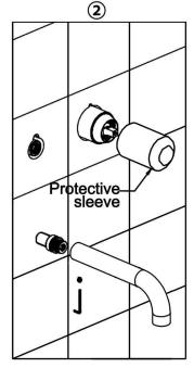
2. Seal the wall, and unscrew the spout as the picture shown.
