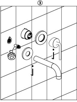
3. Install the part as the picture shown. (wrap the PTFE tape on the thread)
