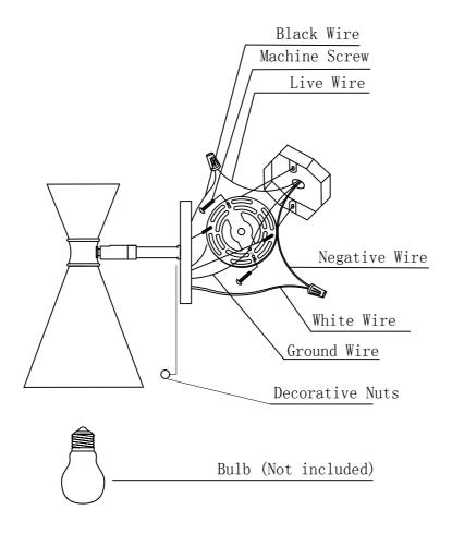
1. Attach the mounting plate to the outlet box by using two mounting screws.
