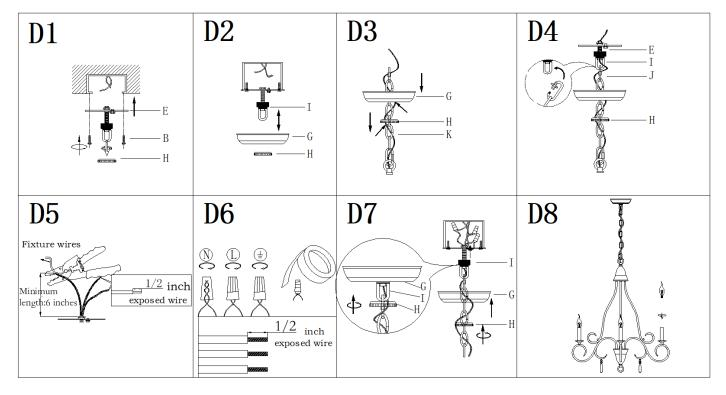
Step D1: .Attach the single bar (E) to outlet box with mounting screws (B). The side of single bar marked "GND" must face out Unscrew the collar ring (H) from the collar loop
