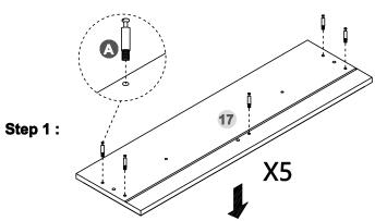
The long groove is used to install the bottom plate, make sure to take note of installing the grooves of these boards on the same side.
